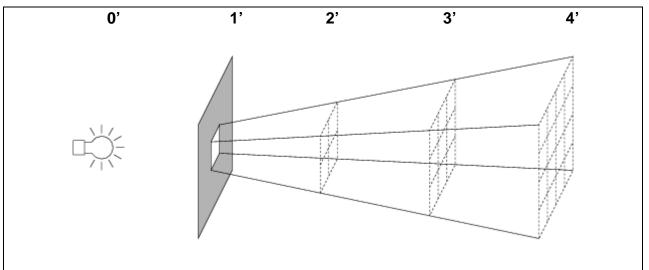
The illustration above demonstrates the inverse-square law. A certain amount of light passes through the hole at a distance of 1 foot from the light-bulb. At distances of 2 feet, 3 feet, and 4 feet from the bulb, the same amount of light spreads out to cover 4, 9, and 16 times the hole's area, respectively (<u>http://www.ifa.hawaii.edu/~barnes/ASTR110L\_F03/inversesquare.html</u>, 3/27/06).
